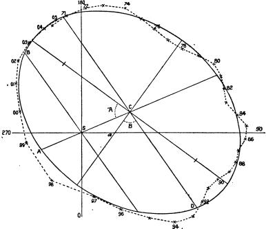
These positions will be found laid off in the accompanying diagram, and an ellipse has been drawn to represent the adopted apparent orbit. The angles should be corrected for precession, viz.:
