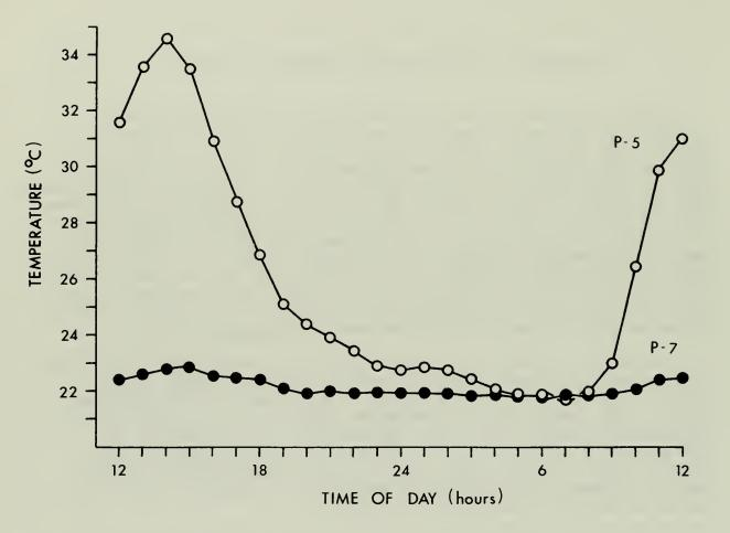
Figure 1. Diel cycle of water temperature (1) in a natural section of stream channel ( $\bullet$ ), and (2) after flowing through 2400 m of concrete lined channel ( $\circ$ ). (From Hathaway 1978).
